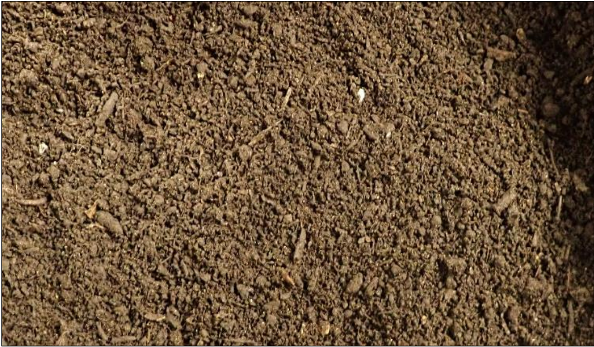
Figure 3. Visual presentation of the contents of composting reactor 1 with Non-wood plant fiber products (0.3 mm; 280 g/m 2 ), cut into 2.5 cm x 2.5 cm pieces, after 6 weeks of composting at ambient temperature
