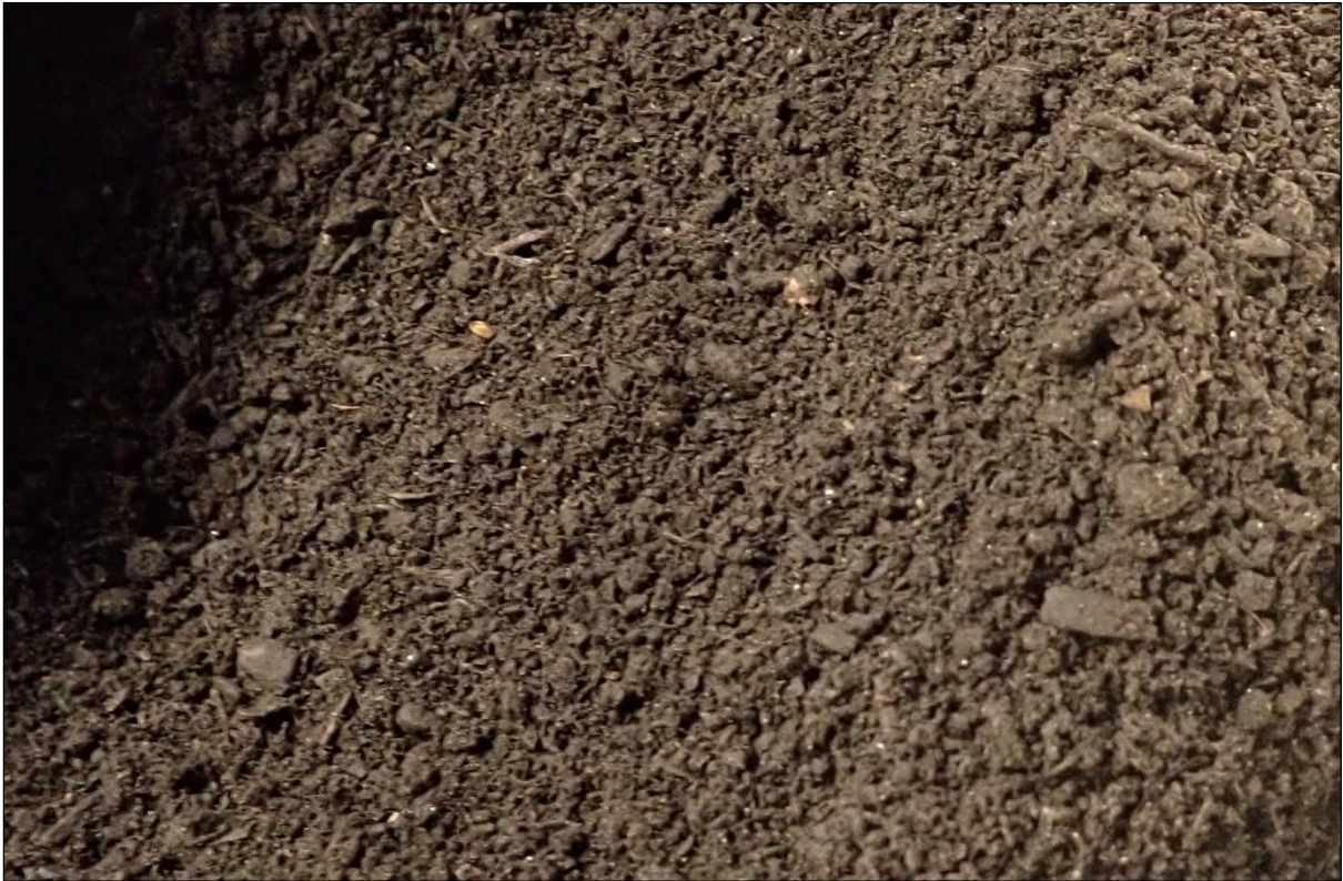
Figure 5. Visual presentation of the contents of composting reactor 2 with Non-wood plant fiber products (0.36 mm; 280 g/m 2 ), cut into 2.5 cm × 2.5 cm pieces, after 11 weeks of composting at ambient temperature
